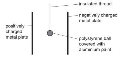
The ball oscillates between the two charged plates.
