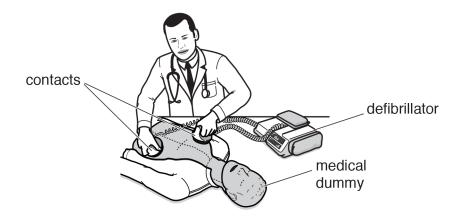
The contacts that touch the dummy are made from metal, and when the defibrillator is being used, one contact becomes strongly negatively charged and the other contact becomes strongly positively charged. The handles of the contacts are made from plastic, which is an electrical insulator.
