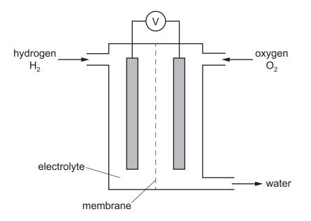
In a hydrogen fuel cell, the hydrogen molecules are converted into hydrogen ions,  $H^+$ , according to the ionic half-equation shown.
