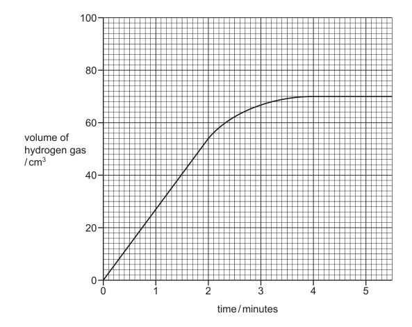
The graph shows the results using small pieces of zinc and dilute hydrochloric acid.
